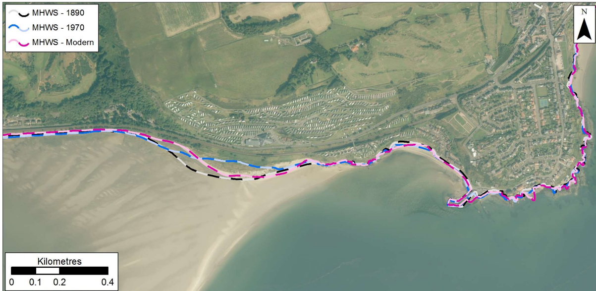
Figure 1.21: MHWs position in 1890, 1970s, and Modern datasets at Kinghorn. Getmapping are our current providers of Scotland-wide digital aerial imagery© Getmapping plc.
