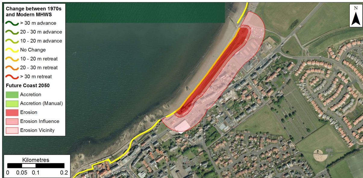
Figure 1.17: Possible future coastline position in 2050 based on rates between 1970 and Modern MHWS data in Prestonpans. Getmapping are our current providers of Scotland-wide digital aerial imagery© Getmapping plc.
