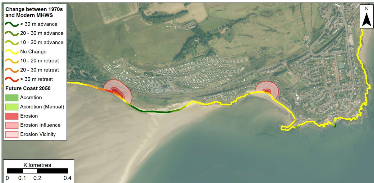
Figure 1.22: Possible future coastline position in 2050 based on rates between 1970 and Modern MHWs data at Kinghorn. Getmapping are our current providers of Scotland-wide digital aerial imagery© Getmapping plc.
