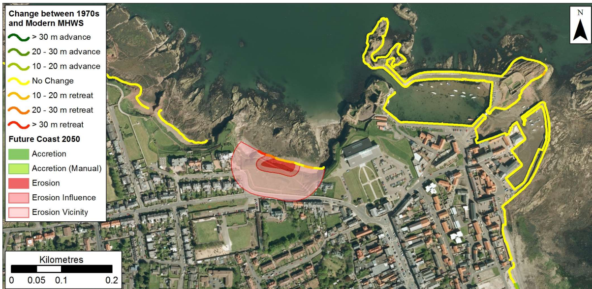
Figure 1.5: Possible future coastline position in 2050 based on rates between 1970 and Modern MHW data. Getmapping are our current providers of Scotland-wide digital aerial imagery© Getmapping plc.
