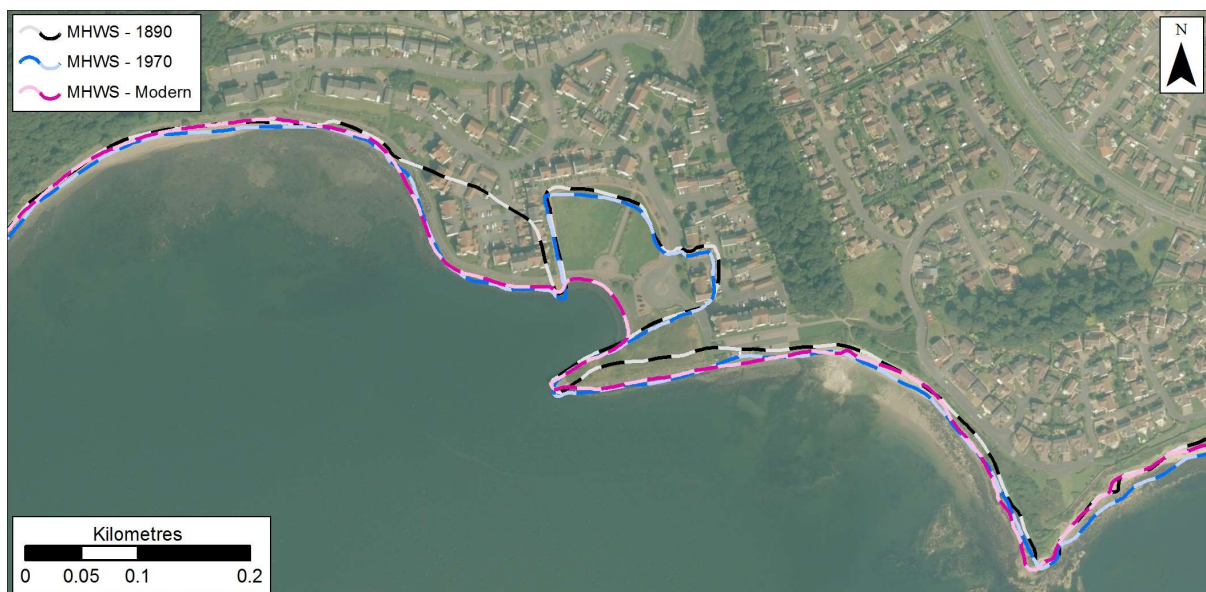
Figure 1.19: MHWS position in 1890, 1970s, and Modern datasets at Dalgety Bay. Getmapping are our current providers of Scotland-wide digital aerial imagery © Getmapping plc.
