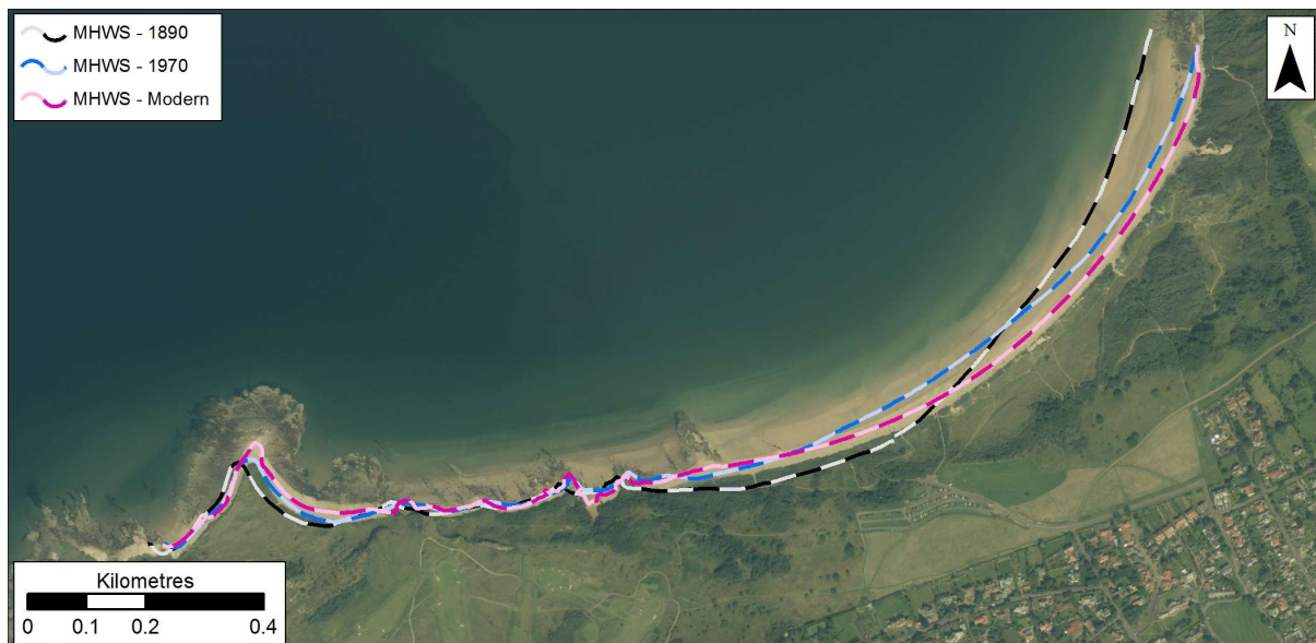
Figure 1.10: MHWS position in 1890, 1970s, and Modern datasets at Gullane Bay. Getmapping are our current providers of Scotland-wide digital aerial imagery© Getmapping plc.
