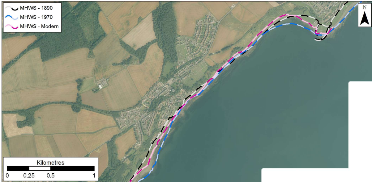
Figure 1.26: MHWS position in 1890, 1970s, and Modern datasets at East Wemyss. Getmapping are our current providers of Scotland-wide digital aerial imagery© Getmapping plc.
